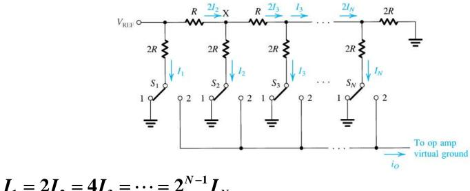
$$I_{1} = \frac{V_{REF}}{2R}, I_{2} = \frac{V_{REF}}{4R} \dots I_{N} = \frac{V_{REF}}{2^{N}R}$$
