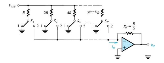
Accuracy of DAC:  $V_{REF}$ , precision of binary resistors, switch performance
