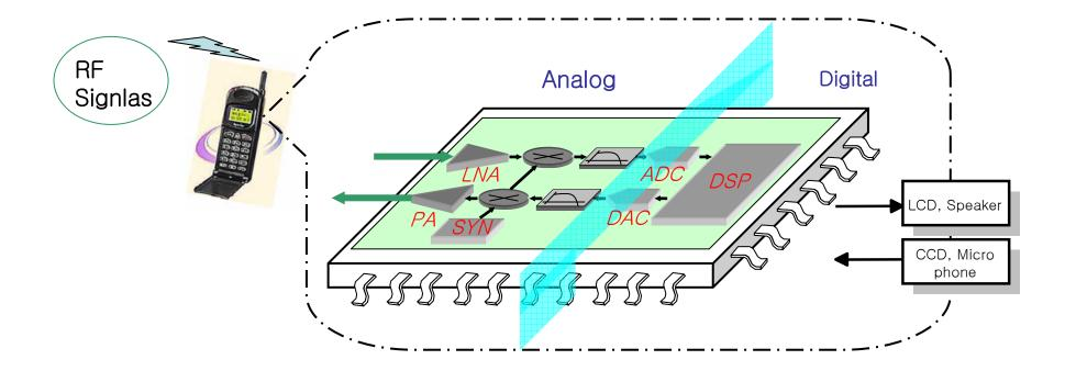
LNA: Low Noise Amplifier PA: Power Amplifier SYN: Frequency Synthesizer
